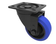
Pressed steel black painted swivel castor with a top plate fixing fitted with a 65 Shore A blue elastic rubber nylon centred wheel with a single ball bearing with retaining caps. Wheel diameter 125mm, tread width 36mm, overall height 156mm, plate size 105mm x 86mm, hole centres 80mm x 60mm. Load capacity 250kg.REACH compliant also PAH-Free rubber to confirm to EU-directive 2005/69/EC
