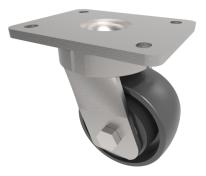
Fabricated swivel castor with a top plate fixing fitted with a cast iron wheel with ball bearings. Wheel diameter 100mm, tread width 50mm, overall height 140mm, top plate 138mm x 110mm, hole centres 105mm x 80/75mm. Load capacity 400kg
