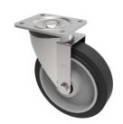
Pressed steel swivel castor with a top plate fixing fitted with a 65 shore A black high elastic rubber on cast iron wheel with ball bearings. Wheel diameter 150mm, tread width 50mm, overall height 200mm, top plate 175mm x 140mm, hole centres 140mm x 105mm; Load capacity 400kg at 4kph, 160kg at 10kph, 150kg at 16kph, 140kg at 20kph \*\* FOR INTERNAL TOWING USE ONLY \*\*
