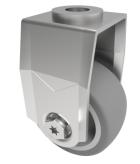
Pressed stainless steel fixed castor with a 12mm bolt hole fitted with a grey thermoplastic rubber tyre on polypropylene centred wheel with Plain Bore. Wheel diameter 75mm, tread width 32mm, overall height 109mm, Load capacity 70kg.
