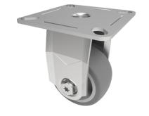
Grade 304 Pressed stainless steel fixed castor with a flate plate fitted with a grey thermoplastic rubber tyre on polypropylene centred wheel with ball bearings. Wheel diameter 50mm, tread width 24mm, overall height 74mm. plate size 60mm x 60mm, hole centres 49.5mm x 49.5mm or 42.5m,m x 42.5mm Load capacity 50kg
