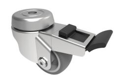
Grade 304 Pressed stainless steel swivel castor with a 12mm bolt hole fixing fitted with a grey thermoplastic rubber tyre on polypropylene centred wheel with a Plain Bore and total lock brake. Wheel diameter 75mm, tread width 32mm, overall height 109mm. Load capacity 70kg.
