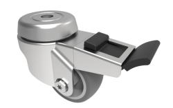
Grade 304 Pressed stainless steel swivel castor with a 12mm bolt hole fixing fitted with a grey thermoplastic rubber tyre on polypropylene centred wheel with ball bearing and a total lock brake. Wheel diameter 75mm, tread width 32mm, overall height 109mm. Load capacity 70kg.
