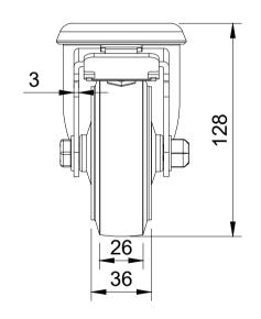
Unspecified Tolerances Machining ± 0.25mm Fabrication ± 1mm
