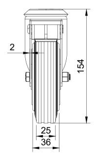
UNLESS OTHERWISE **SPECIFIED** DIMENSIONS ARE IN MILLIMETRES
