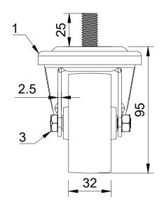
UNLESS OTHERWISE **SPECIFIED** DIMENSIONS ARE IN **MILLIMETRES**
