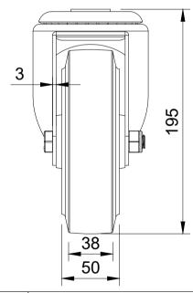
UNLESS OTHERWISE **SPECIFIED** DIMENSIONS ARE IN **MILLIMETRES**
