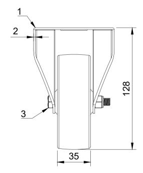
UNLESS OTHERWISE **SPECIFIED** DIMENSIONS ARE IN **MILLIMETRES**
