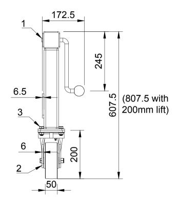
UNLESS OTHERWISE SPECIFIED DIMENSIONS ARE IN MILLIMETRES
